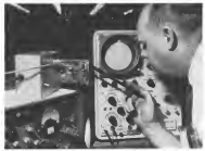
RF HIGHER SPEED, easily visible on scope, reveals an intermittent type fault in subassembly under test. New technique developed by Minneapolis-Honeywell permits detection of solid solder joints and other resistive connections in components and printed wiring boards which could not be discovered by other available techniques.
